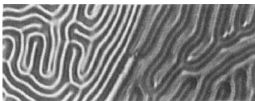
FIGURE 5 The cholesteric texture of 5-CB with 1% of chiral dopant. See Color Plate VII at the back of this issue.
