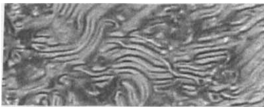
FIGURE 1 The chiral texture of p -octylbiphenylcarboxylic acid. See Color Plate III at the back of this issue.
