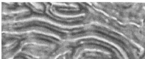
FIGURE 3 Large periodic structure with in-plane period in the smectic C phase of p-octyloxybenzoic acid See Color Plate V at the back of this issue.
